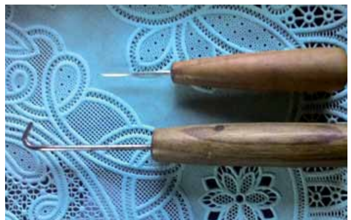
Gantol and tunccek, two indispensable tools for homeworkers to sew shoes, Photo: Dietrich Weinbrenner
